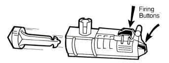
5. Insert top peg of launcher into slot on bottom front of grabber and rotate up to locking position.
