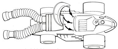
3. Insert windshield pegs into holes in body.
